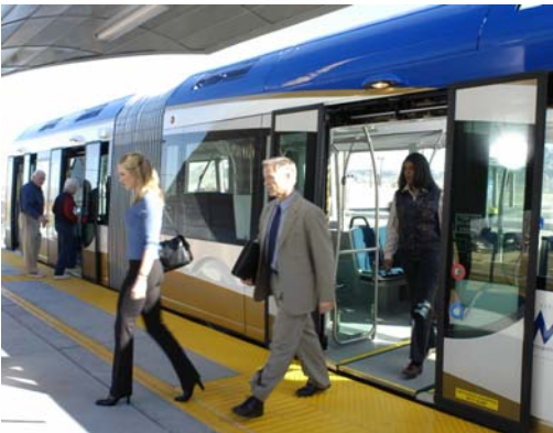
Boarding on Las Vegas' MAX bus rapid transit system is significantly faster than on its regular buses. MAX's delay-reducing features include off-vehicle fare payment, level boarding, and buses with multiple doors. Photo courtesy RTC of Southern Nevada.
